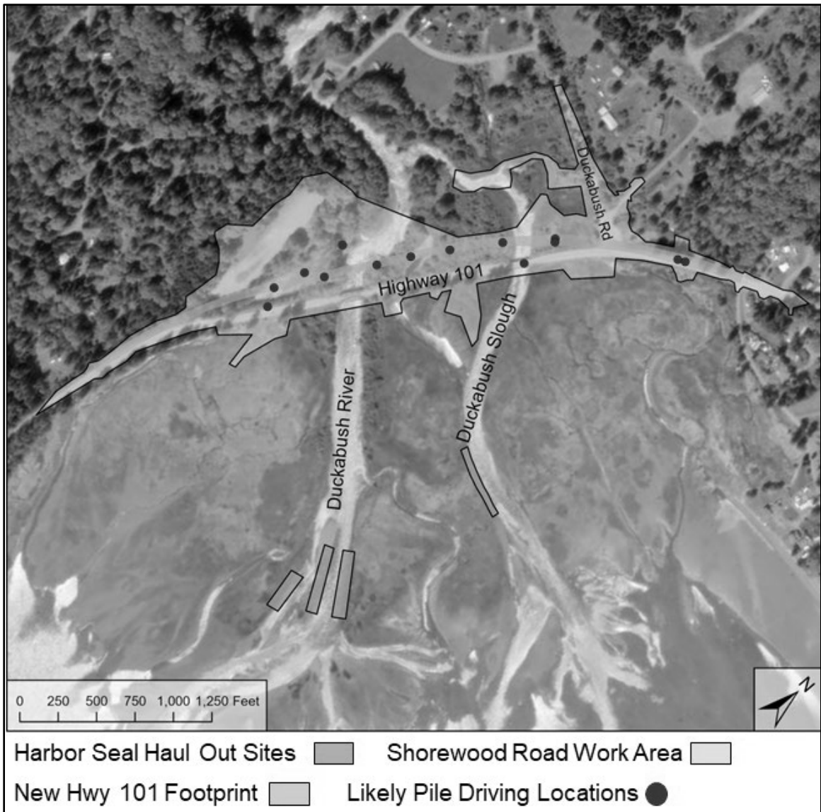
Figure 1. Project Site Including Likely Pile Driving Locations Relative to Harbor Seal Haulout Sites
