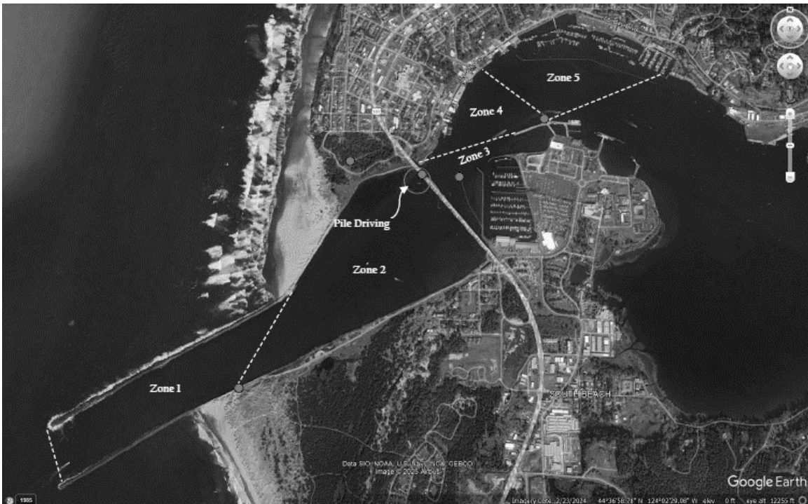
Figure 2 – Proposed PSO Monitoring Locations (Gray Dots) During Vibratory Pile Driving Activities for the Yaquina Bay Dolphin Replacement Project.
