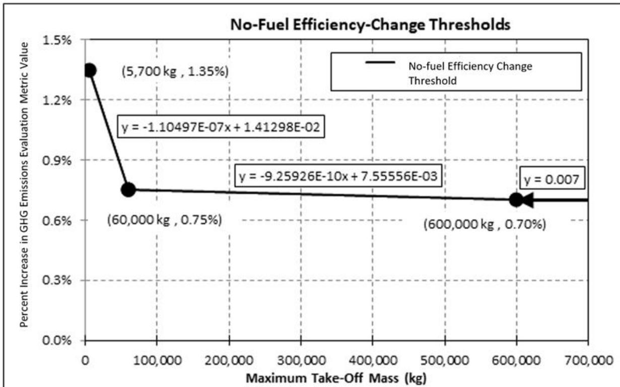
**Figure IV-5: No Fuel Efficiency Change Thresholds for GHG Certificated Airplanes (ICAO Adopted No CO<sub>2</sub> Emissions Change Thresholds)**
